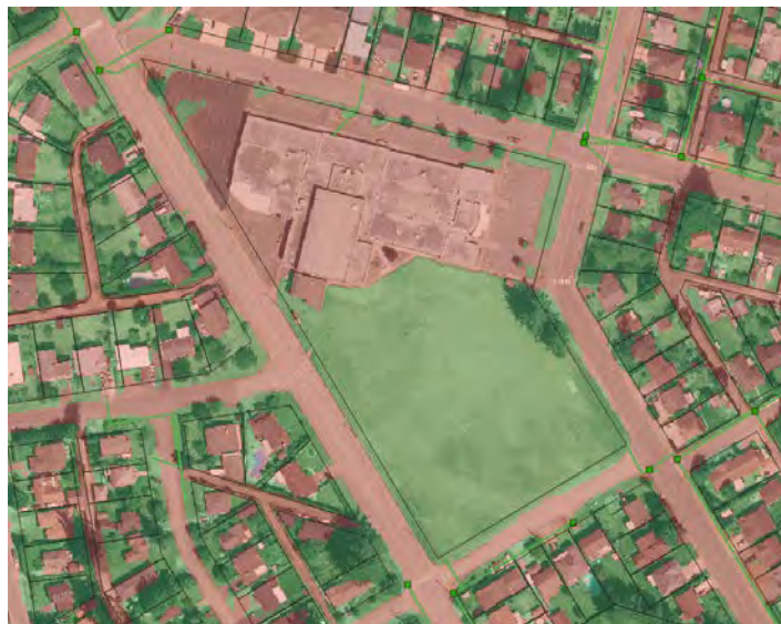
FIGURE 2-2: TYPICAL OUTPUT OF GIS SOFTWARE IMPERVIOUS AREA ALGORITHM – RED = IMPERVIOUS, GREEN = PERVIOUS
