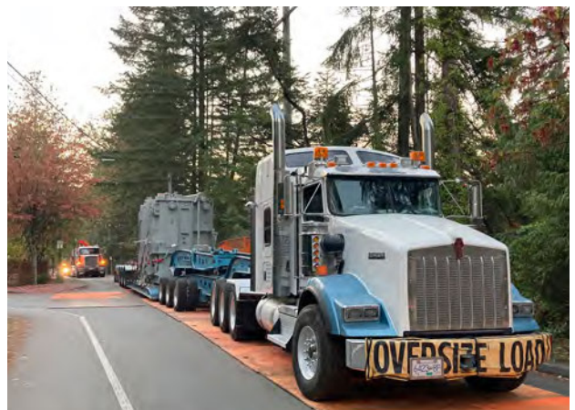
The delivery truck carrying the transformer. The specialized truck and trailer has 13 axles and 50 tires to spread out the load and reduce contact pressure on roads and bridges. The truck carried the transformers – one at a time – from the port in Everett, Washington to a drop-off point in North Vancouver.
