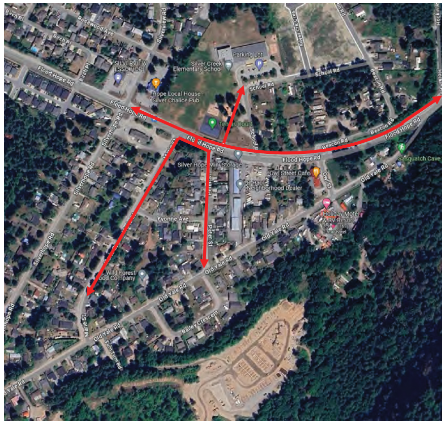
Figure 4: Pedestrian Desire Lines (Silver Creek Area)
