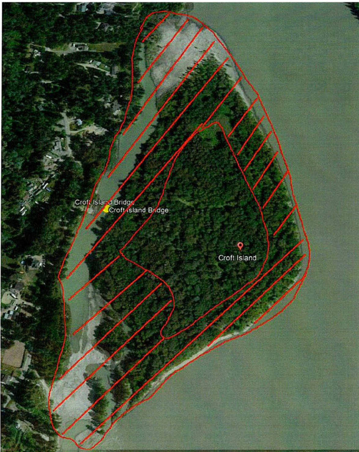
Image 3. Stop Work Order S.93 Boundary. The red shaded area is the area where works are not permitted i.e. within 30 m of the Top-of-bank or High-water-mark, whichever is higher.
